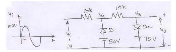
2 A clamping circuit and input wave form is shown in figure 2b calculate and plot to scale the steady state output
