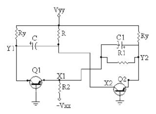
9. (a) The fixed-bias bistable multivibrator uses n-p-n transistors with  $h_{FE} = 20$ . The circuit parameters are
