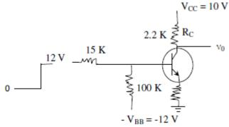
6. Prove that the circuit show works as a transistor switch. Assume junction voltage and  $(h_{FE})_{min} = 30$ .
