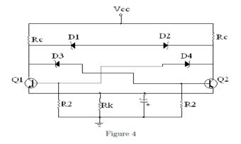
2. (a) Consider the symmetrical emitter triggering circuit of the figure 4 with Rc=3Re, R1=2R2, and Vcc=6V. Indicate all the circuit voltages in the quiescent state and indicate also the voltages immediately after a 5-V positive step is applied. Assume that D3 and D4 are always in the breakdown region and that either D1 or D2 but not both in the breakdown region.
