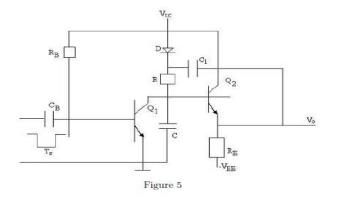
4. (a) With the help of a neat circuit diagram and waveforms explain the working of a transistor Miller time base generator.
